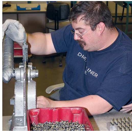
Robert Peterson performs the “pressing” operation for rivet assembly.
